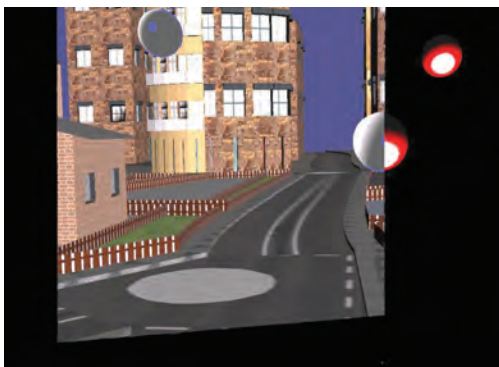
Illustration 3: Experimenting pre-attentive vision in a telepresence environment : the user's visual focus is monitored while presenting him attentional audio-visual stimuli in the EVE system. Note that because of the actual teleoperation setup, no peripheral vision is transmitted back from the remote vehicle to the subject. Nevertheless on-board processing can detect such "early warnings" and send them back to the VR supervisor.
