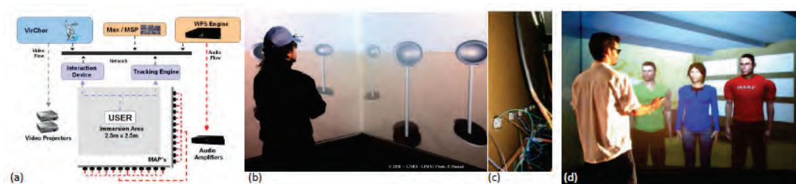
Illustration 2: SMART-1 2 (a) architecture, (b) view from the user perspective, and (c) rear view of actuators. (d) Virtual characters of the MARC platform (developed by groups AMI and CPU) for real-time affective interaction integrated into SMART-1 2 .
