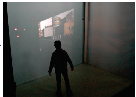
Illustration 3: Experimenting pre-attentive vision in a telepresence environment : the user's visual focus is monitored while presenting him attentional audio-visual stimuli in the EVE system. Note that because of the actual teleoperation setup, no peripheral vision is transmitted back from the remote vehicle to the subject. Nevertheless on-board processing can detect such "early warnings" and send them back to the VR supervisor.
