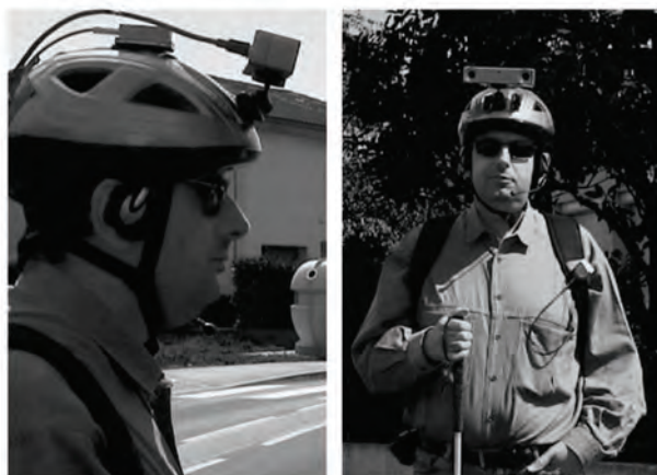
Illustration 2: the NAVIG prototype including a GPS receiver, a stereoscopic camera, and a head motion tracking device mounted on a helmet. Microphone and headphones are used to transmit speech and audio information.
