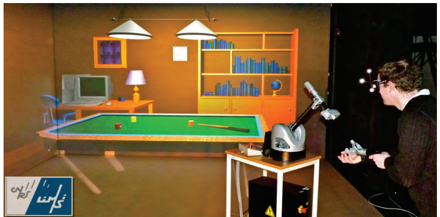
Illustration 2: Interactive simulation of a relativistic carrom billard game in the EVE system : the user shoots a ball at a speed close to the speed of light thanks to a haptic interface and observes its interactions with other balls in the 3D scene (cf. ANR "EVEILS" project – topic 2)
