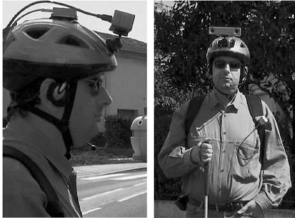
The NAVIG prototype including a GPS receiver, a stereoscopic camera, and a head motion tracking device mounted on a helmet. Microphone and headphones are used to transmit speech and audio information.
