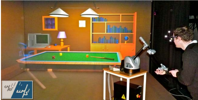
Illustration 1 - Interactive simulation of a relativistic carrom billard game in the EVE system: the user shoots a ball at a speed close to the speed of light thanks to an haptic interface and observes its interactions with other balls in the 3D scene (cf. ANR "EVEILS" project – topic 2)
