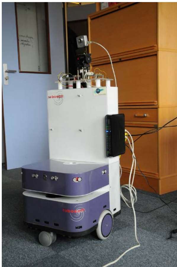
The robot (Robulab 10 from Robosoft) used at LIMSI for place and object recognition and autonomous navigation experiments
