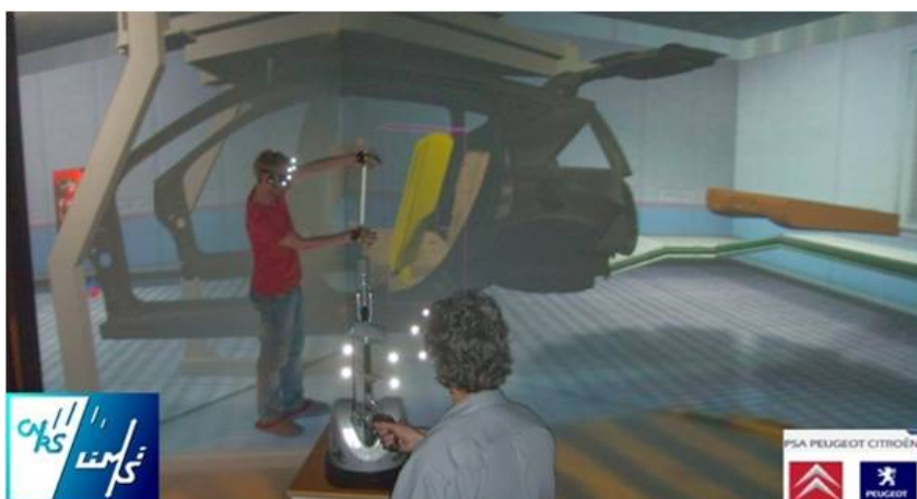
Illustration 2 – MaCoMIICs (Multimodal and Co-localized Multi-user Interactions for Immersive Collaborations): In a virtual assembly chain, two users cooperate in the EVE system with speech, two-hand gestures, haptic feedbacks, and double-stereoscopy to define the trajectory of a seat which must be set in the cockpit of a car (cf. Digiteo "SIMCoD" project – topic 1).
