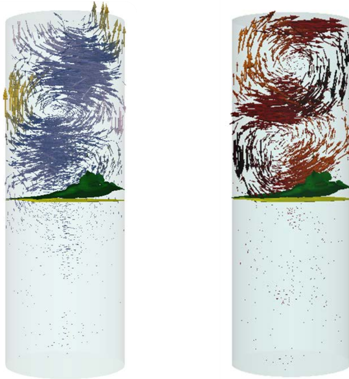
Figure: Velocity (left) and perturbed current (right) fields in a modeled Liquid Metal Battery (LMB) near short-circuit. The Taylor instability in the top liquid electrode has generated two counter-rotating vortices strong enough to wash away the fine electrolyte layer between the two electrodes. The yellow surface is the interface between the electrolyte and the bottom liquid electrode, the green surface is the interface between the electrolyte and the top liquid electrode. Results from SFEMaNS (2014)
